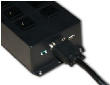
3. Plug the temperature probe to the head unit
