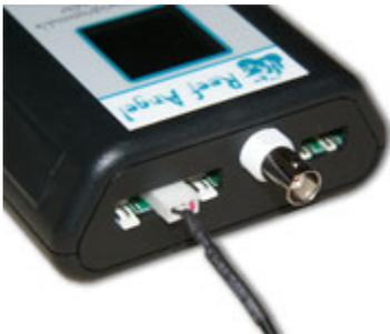
4. Plug the pH probe to the head unit
