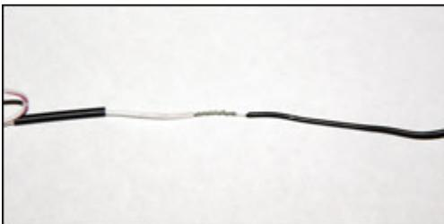
Twist the wires together.
