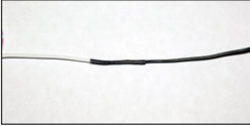
Apply heat to the shrink wrap tubing.
