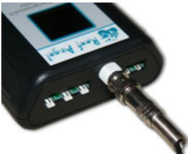
5. Insert the power cord to the power inlet connector of the relay box.
