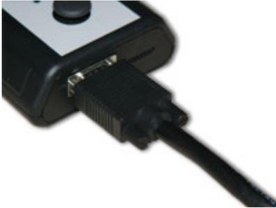
2. Insert the other end of the communication cable to the communication connector of the relay box.
